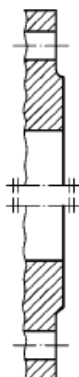
Tipo / type B Tenuta a gradino (B1 e B2) Raised face (B1 and B2)
