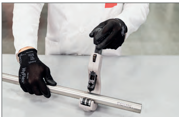
Taglio del tubo / Cutting the pipe to length
